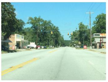
Roadway design doesn't typically change to account for potential non-motorized traffic through population centers in Colleton County. For example, the roadway pictured is wide to cross and only has sidewalks on one side. This type of design is unsafe and discouraging to bicycle and pedestrian traffic. (location: Alternate 17, Cottageville)
