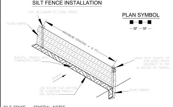
SILT FENCE - GENERAL NOTES not be used as a velocity control BMP. Concentrated flows are any flows greater than 0.5 cfs.
