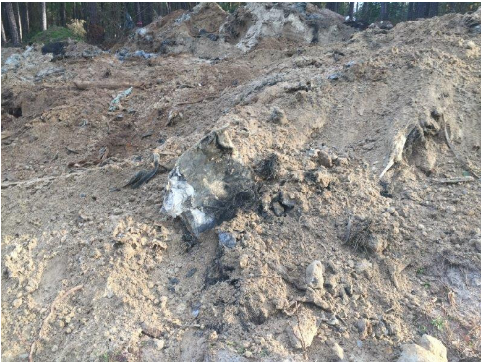
Photograph 2: View of the suspect waste oil drum within Test Pit 1.
