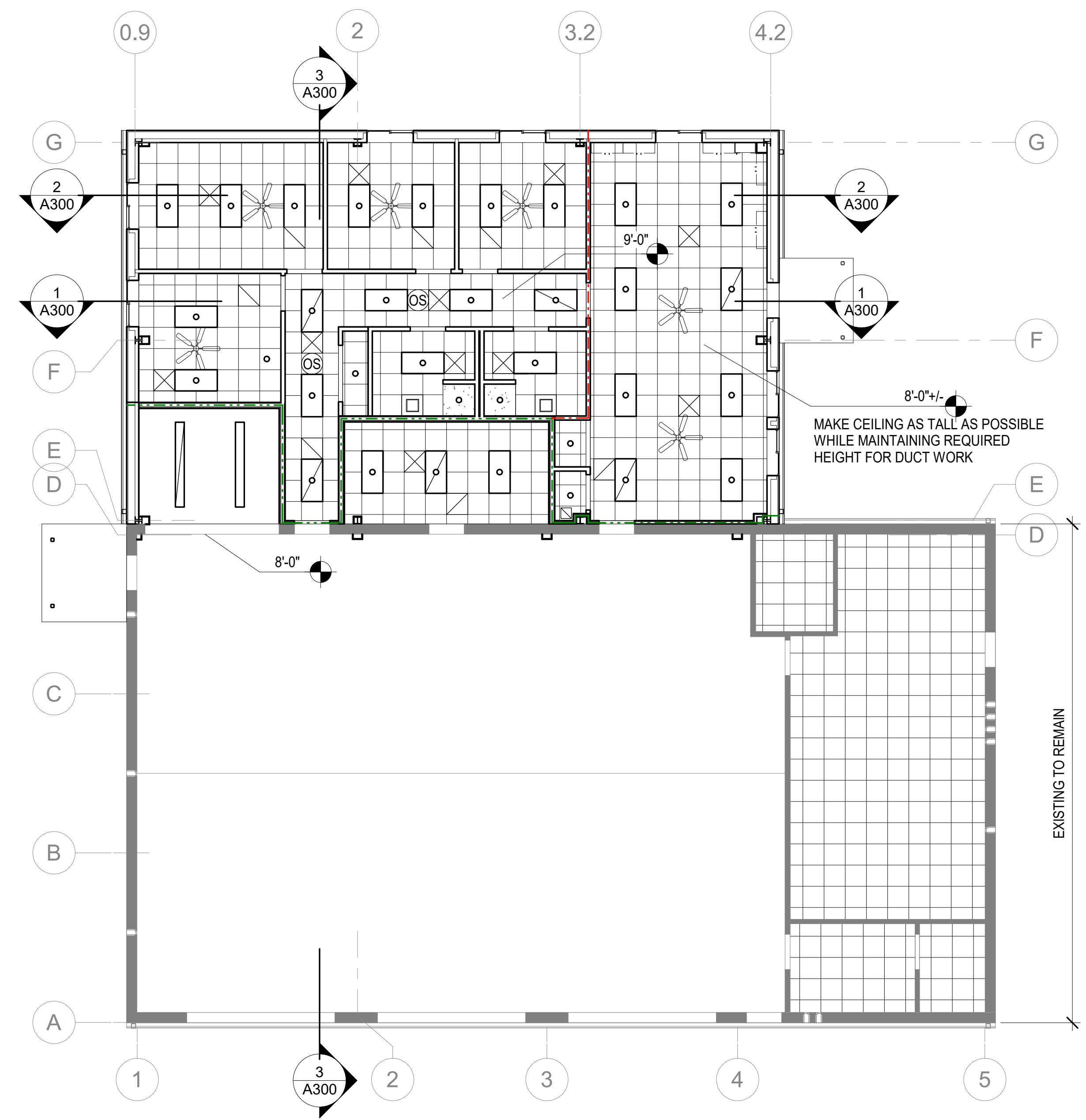
2 FIRST FLOOR REFLECTED CEILING PLAN A101 SCALE: 1/8" = 1'-0"
